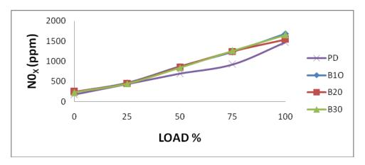
Fig 4.6: Variation of NOx with respect to load
