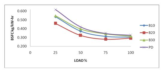
Fig 4.1: Variation of BSFC with respect to load
