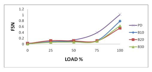
Fig 4.7: Variation of smoke with respect to load
