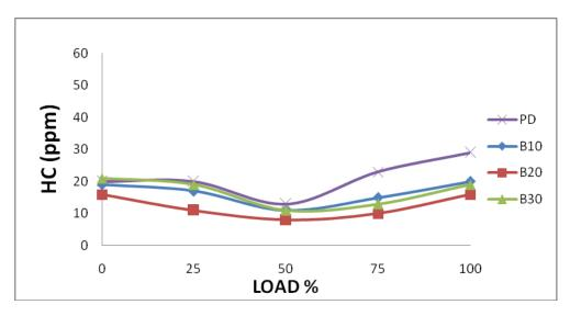
Fig 4.5: Variation of HC with respect to load
