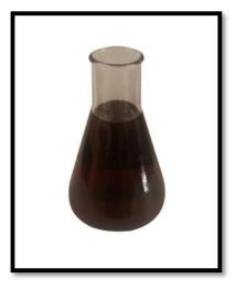
Fig.3 Waste Transformer Oil
